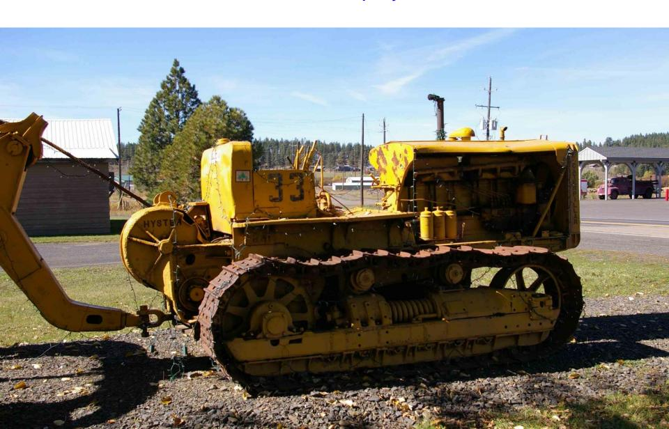
7- This view of the logging arch shows the cable and chains used to lift the end of the logs.
