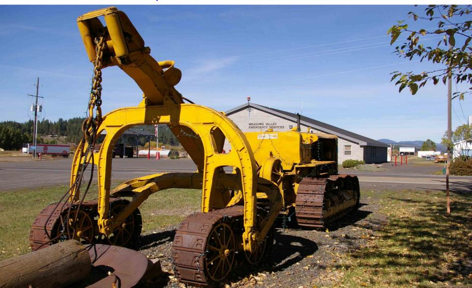
4- The "pan" behind the arch does not appear in any photos I found of working logging arches. Proper operation of the arch should keep the log from "plowing" a furrow even without the pan.
