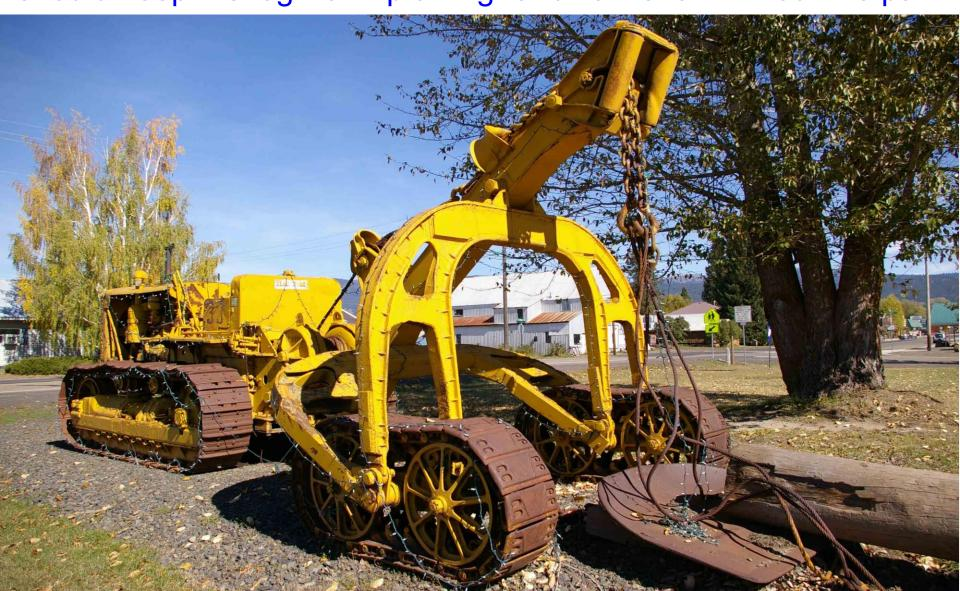
5- This side view of No. 33 shows the Hyster cable winch and control levers, which are very similar to the ones found on the GHQ model.
